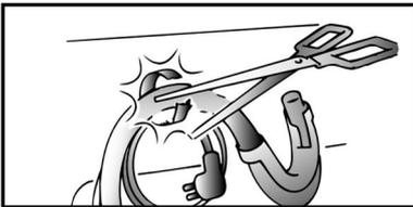
Carefully cut through the hose retaining clip at the rear of the appliance (diagram 1).
